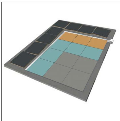
Begin replacing the previously flipped tiles, connecting the back of the tiles to the half-exposed tape. Start at the outside edge.
