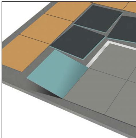
Flip all tiles that adjoin the anchor tiles backing side up. Move them away from the anchor tiles to allow room for taping.
