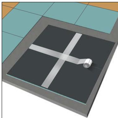
Begin in a corner by flipping four tiles backing side up.
