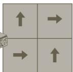
During installation, rotate tiles so that arrows are turned 90 degrees every other tile.
