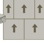
Offset the side joints of the tiles with arrows facing in the same direction.
