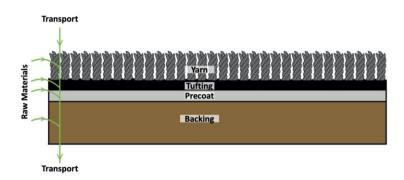
A1-A3 measured flows include manufacturing processes, transport, and raw material inputs for each product layer and sub-layers.
